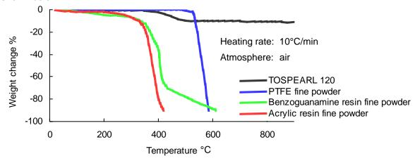
Differential thermal analysis date of TOSPEARL 120 and PTFE fine particle are shown below.
